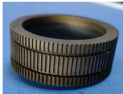
Figure 7.2 Left – rotor armature with 90 teeth. Right – Double-stack rotor with permanent magnets.
