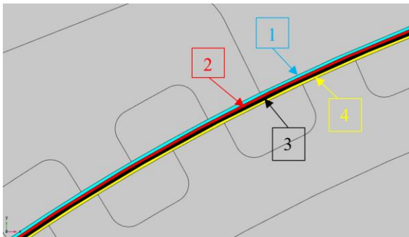
Figure 6.1 Division of the air gap into cylinders of equal volume.
