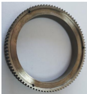
Figure 7.2 Left – rotor armature with 90 teeth. Right – Double-stack rotor with permanent magnets.
